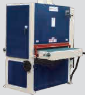
43x75 Double Head Mechanical Tracking Line Shaft Shown with Factory Installed Clutch
